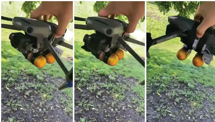
DJI Mavic 3 modified by Ukrainian fighters to carry two M433 40mm grenades. 17
