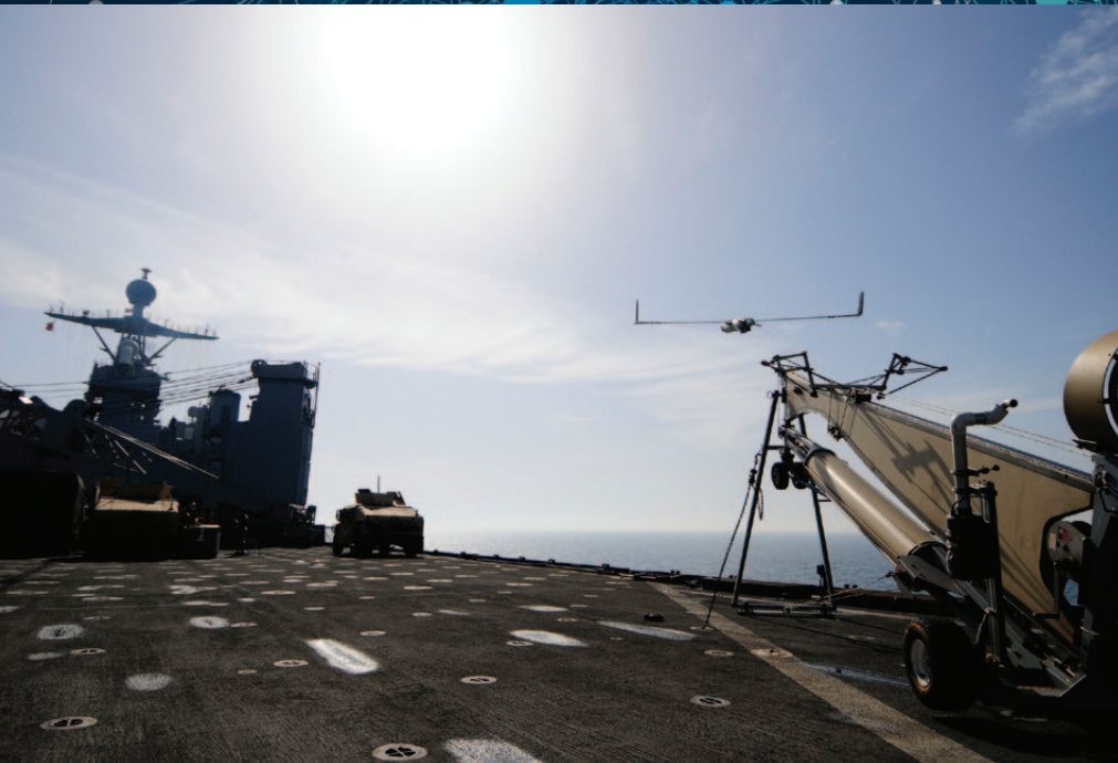
A ScanEagle unmanned aerial vehicle launches from the flight deck of the dock landing ship USS Comstock (LSD 45) in the Persian Gulf May 17, 2011. Comstock is supporting maritime security operations and theater security cooperation efforts in the U.S. 5th Fleet area of responsibility. (U.S. Navy photo by Mass Communication Specialist 2nd Class Joseph M. Buliava/Released)
